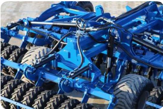
*Châssis repliable hydraulique*
